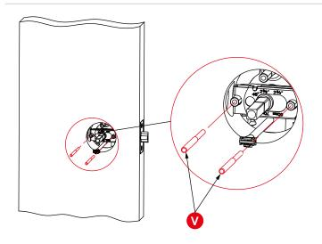
Insert Positioning Rods Vinto the holes to the left and right of the Spindle ©. The holes are located at the 3 o'clock and 9 o'clock positions.
