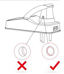
Confirm that your installation was complete by checking if the pins are flush against the handle, and has popped out. Adjust the handle accordingly to make sure the pins are fully decompressed and sits flush against the surface.
