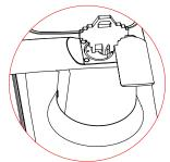
Twist key back to horizontal position. The key can be taken out once it goes back to the horizontal position.
