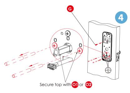
Remove the position rods **V** and replace them with screws **O** Tighten clockwise until the mounting plate is secure.
