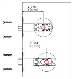
Facing the door exterior, install the lockset according to the in-swing or out-swing opening direction of your door.
