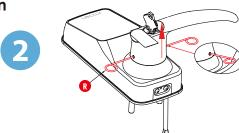
Use the provided pin insert **R** to push the metal pin located at the 3 o'clock of the the base handle, then the other pin at 9 o'clock position. Remove the handle once the pins are compressed.
