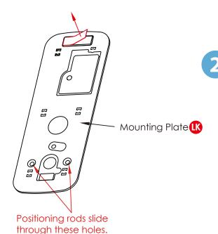
Interior Mounting Plate will go against the interior side of your door. Remove the paper layer off of the Adhesive Tape and align the positioning rods on the bottom of the plate to the corresponding left and right holes.
