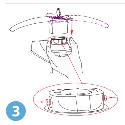
Rotate the handle 180° to the other side of the lock.
