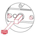
Pass the Spindle 6 through the center of the lockset, and the round rods through the sides in their respective holes. The cable should run underneath the lockset.
